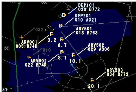
B. Display of distance between the runway edge and the arrival aircraft
